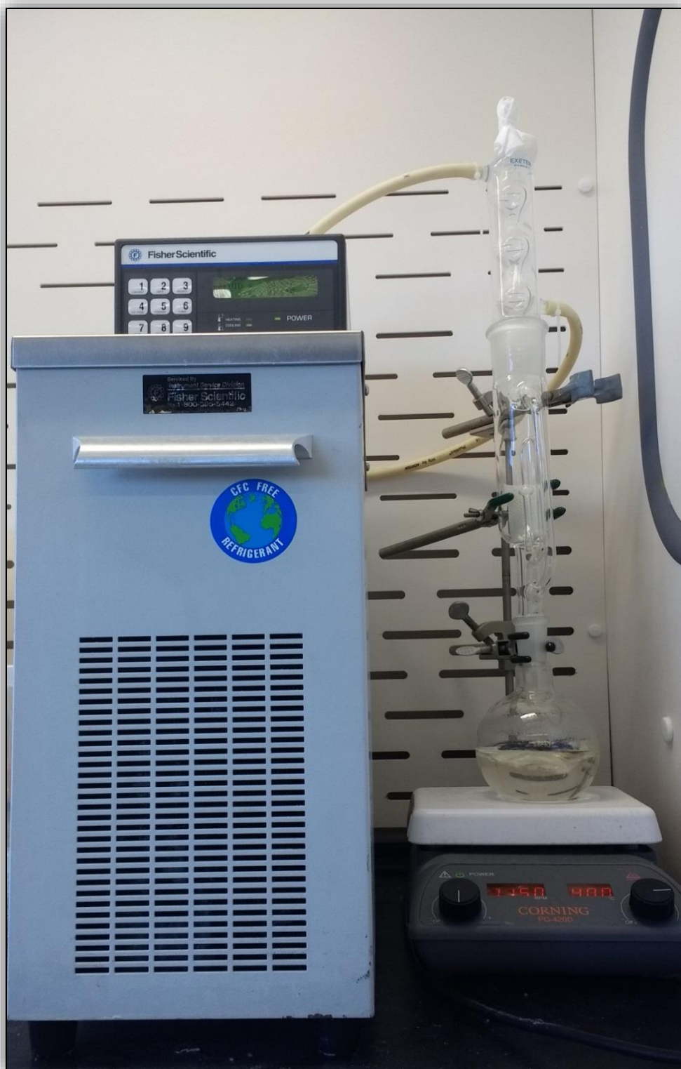
Figure 3.10 Soxhlet extractor used in the experiment for cleaning process
