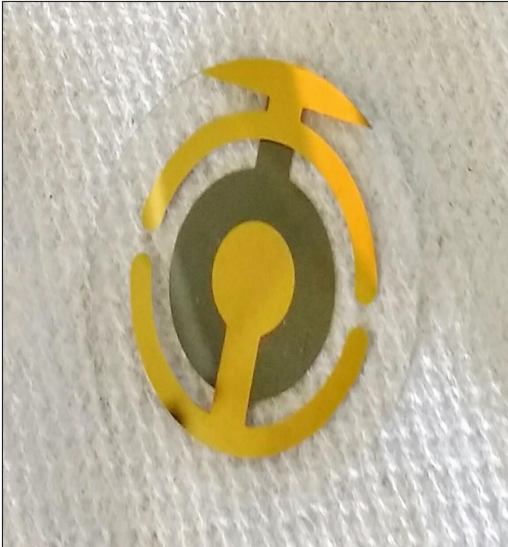
Figure 3.2 Quartz crystal used in the experiments (rear)
