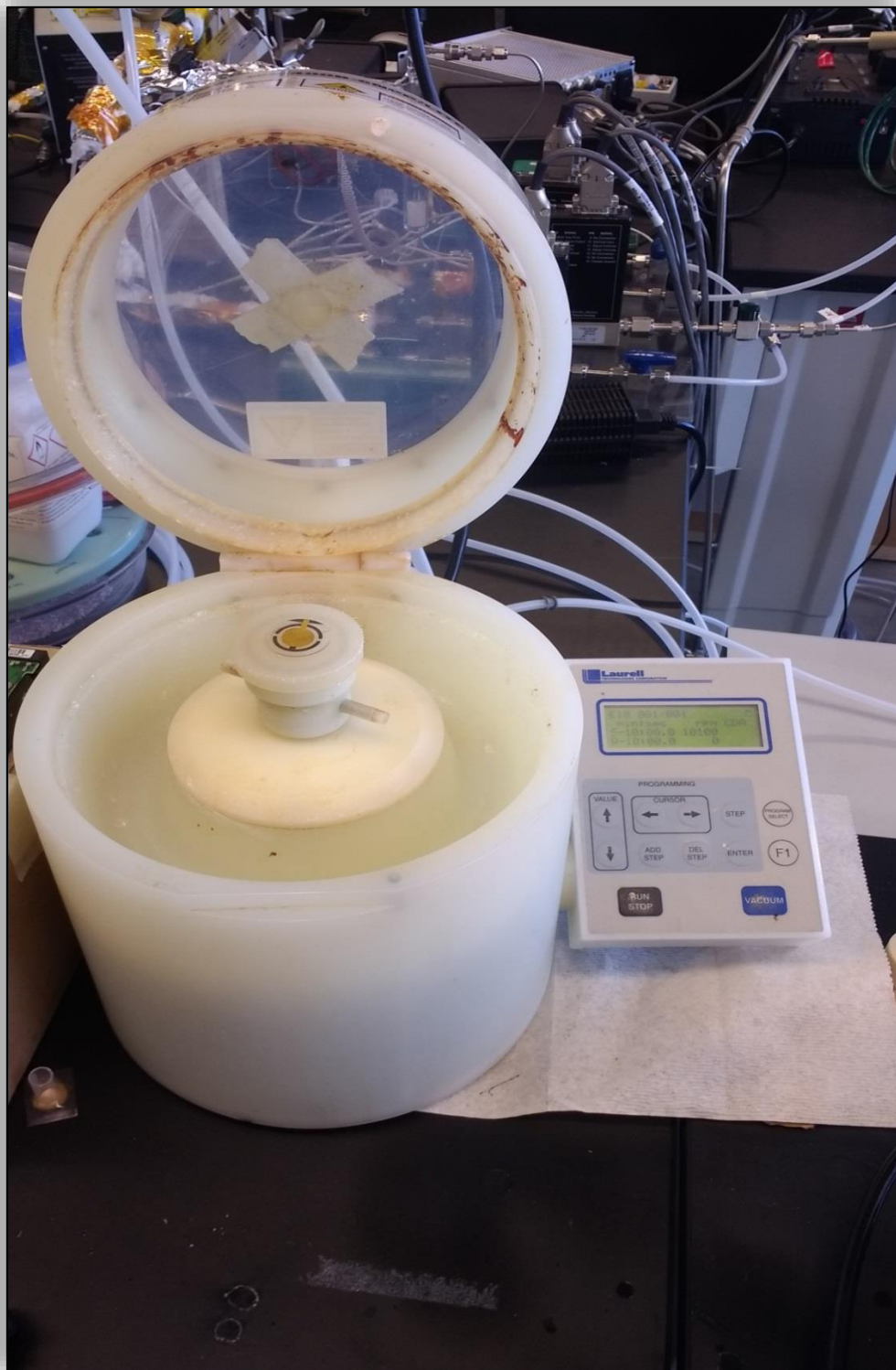
Figure 3.11 Spin coater for the polymer coating on the cell
